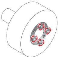
Loosen the clamping screws slightly if necessary. Position the Posi-Lok assembly to the desired location, making sure both the shaft and the hub engage the full length of the bushing. Hand tighten each clamping screw lightly to gently grip the hub and shaft.
