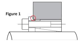
bushing, that the hub engages the full length of the bushing sleeve, and that the flange pilot is in tight contact (no space) with the end of the hub (see Figure 1).
