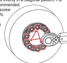
Make a final tightening of all clamping screws in a sequential pattern to the specified torque using
