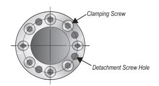
Caution: The Posi-Lok bushing is designed to release immediately when clamp screws are loosened
