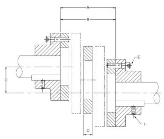
Position shafts and hubs according to the following values:
