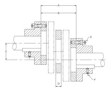
Position shafts and hubs according to the following values:
