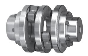
• C: Maximum shaft misalignment not to exceed: 0.313 inch Note: The Schmidt Inline Coupling cannot operate properly at higher misalignment than listed. For speeds over **1000 rpm**, maximum shaft misalignment should not exceed **0.060 inch**.
