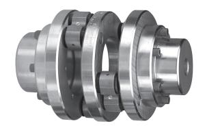
• C: Maximum shaft misalignment not to exceed: 0.188 inch Note: The Schmidt Inline Coupling cannot operate properly at higher misalignment than listed. For speeds over 1000 rpm, maximum shaft misalignment should not exceed 0.060 inch.
