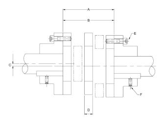
Position shafts and hubs according to the following values:
