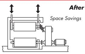
Diagram overcomes both problems by the use of a Schmidt Offset Coupling.
