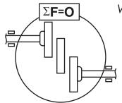
Wide range of parallel shaft displacement without sideloads
