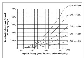
The graph shows the InLine /5D coupling's reaction to parallel misalignment. Machinery sensitive to sideload forces generated by the coupling may require closer shaft alignment. Machinery not sensitive to sideload forces may allow for more misalignment than shown in the dimension and performance data tables.
