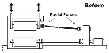
Diagram shows how this can be achieved with double universal joints but causes radial forces at the joints and requires large lateral space.
