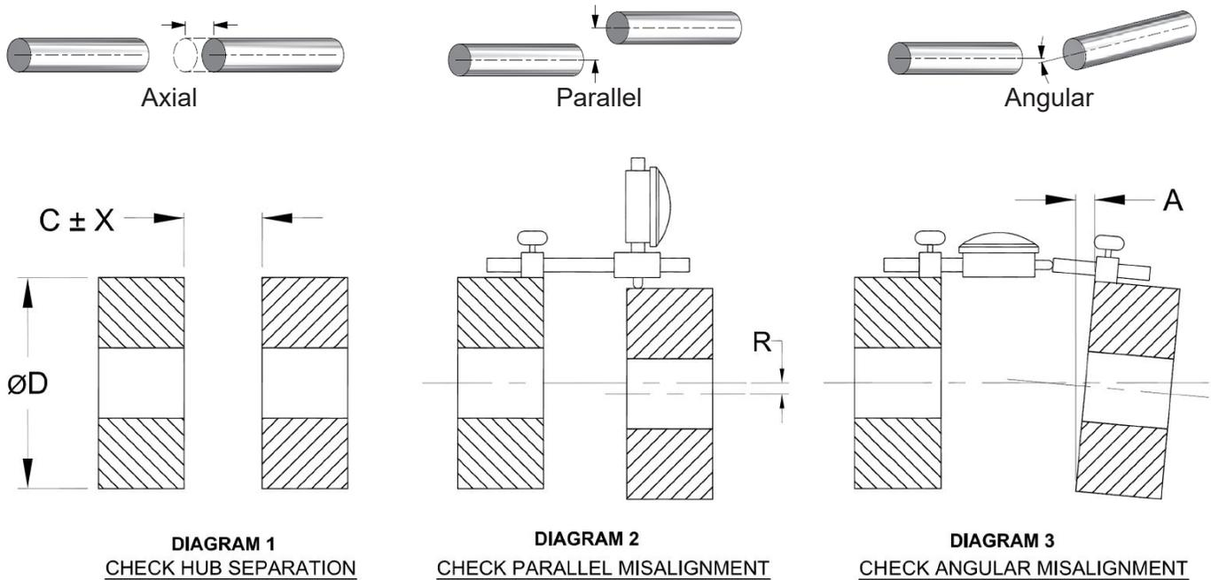
**Table 1: Alignment and Assembly Specifications for Single-Flex A1C Couplings.**
